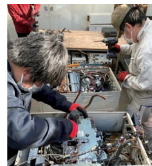
給湯器解体①
